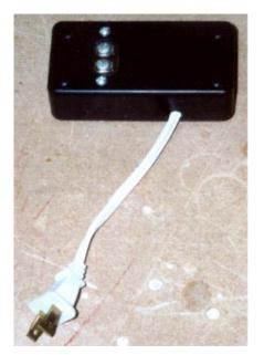
I just cut a slot out of one side of the box, drilled two holes and mounted the attachment board facing out. I also had to grove a hole out from between both top and bottom sections to get the power cord out. Now we are ready to put this to use.
