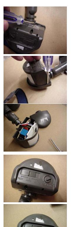
Place a small screwdriver in-between the case and the lid and pry back a little. There is a little catch that needs to be released.
