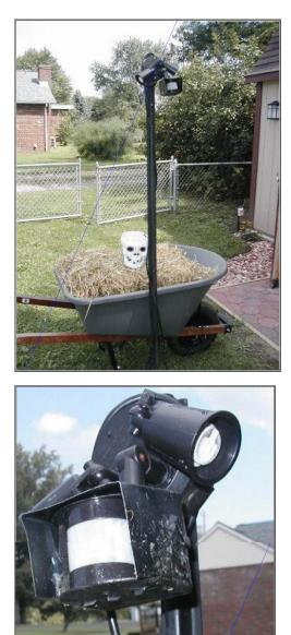
We use a simple floodlight motion sensor to trigger some of our yard haunt lighting and effects when a visitor drives by our display.
