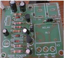
Q2 is BC547 It too is marked "C547B" and Flat sides must line up
