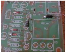
D3 & D4 are 1N4004 Power diodes. Strip must go towards the Direction the arrow is pointing.
