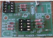
Be sure the notch in the middle of the socket is facing the same way as drawn on the board. This will be important when install the chips later.
