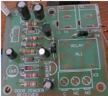
Q3 is BC557 on the component itself it is sometimes marked like this though "C557B" Make sure the flat sides on it and the board line up
