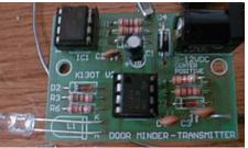
The chips have a dot in the middle on one side be sure that you put the chips in with the dot towards the notch in the socket. you may need to bend the pins in just a little to allow them to slide into the socket.
