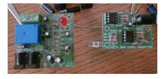
This Kit uses an infrared beam to monitor door & passageways or any other area. When the beam is broken a relay is tripped which can be used to sound a bell trip an effect or cut off one. Suitable for detecting customers/victims, cars ect.
