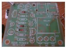
Bend the restores and diodes in a U shape now to save time.
