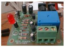
X3 is the terminal block. be sure the holes are facing out. Believe me it can happen (don't ask). Receiver Board is now DONE
