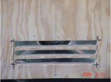
A grill was cut unobtrusively in the bottom part of the front; this is where the lowlying fog will exit.
