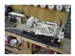
The tan box to the left of the skeleton's head is the PLC I am using to continuously cycle (stress test) this guy.
