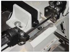
Cutting off the tail flush with the housing around the bleeder adjustment screw.
