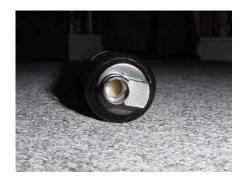
If you try to use a large bit you'll just tear up the end of the closer. I started with a bit that was just slightly larger than the bleeder hole and worked up to drill size "R". Then I ran the 1/8"NPT tap through it.
