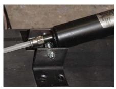
Here it is mounted. The tubing just pushes into the end of the fitting. Just cut it to length and push it in. Depending on material and manufacturer, these fittings will cost between \$1.00 and \$2.50. They are also available with a 90 degree elbow and other configurations. (costs more)
