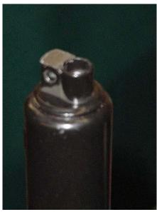
I found I did not need to tap the hole. The threads cut their way into the relatively soft aluminum housing.
