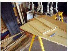
After the lid and bottom are dry measure out the exact dimensions of the coffin and mark them. I measured a line from the middle of the board to make sure I was centered.
