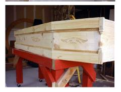
Next rip the last 6'-0" board into four equal lengths it will be used on the coffin around the top and bottom edges.
