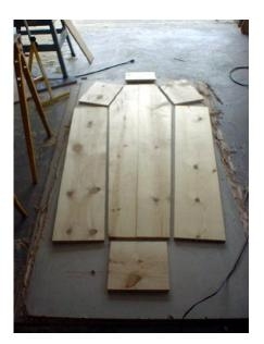
Here are all of the pieces laid out prior to assembly. All the joints are cut to either a 5 or 20 degree, most of these I eyeballed but hey that's what wood putty is for!!
