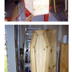
Here is my finished lid with all the trim and molding on it I used wood putty to fill any gaps and smooth joints.
