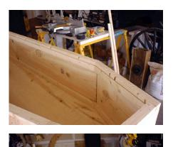
Next I used 1x4 stringers attached to the top lip this gave me another 3/4" in depth and a nice smooth finish to rest the lid. You can see this in the picture below. Now make an identical frame work matching the one on the lip of the coffin to attach to the lid this part was very tricky mine had to be exact because my finished lid will fit inside a trimmed edge.
