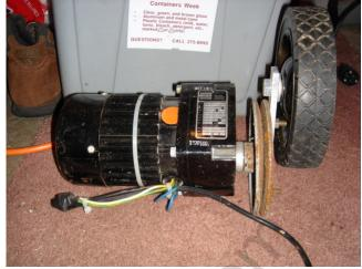
The first step is finding a motor that handle this type of load. The motor that I used was Bodine 1/15 hp with 10 RPM motor from C & H Sales Company. You can find them in my Links page. This motor has a 5/8 shaft and also has a hole drilled through the shaft. The arm is a piece of aluminum that is ¼ inch thick and 7 ½ inches long. The arm attaches to the motor using a 5 inch diameter V-belt wheel. The other end of the arm which opens the lid has a 6 inch lawn mower wheel attached to it.
