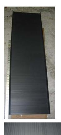
On the three 4' x 16" side pieces place a score line 1" in from each side running the length of the piece. Once scored, the piece was bent to create a 90 degree bend. When scoring take care as not to cut all the way through the plastic.
