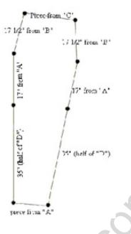
This sketch shows how to cut the A, B, C, and D pieces so they will fill around the coffin bottom
