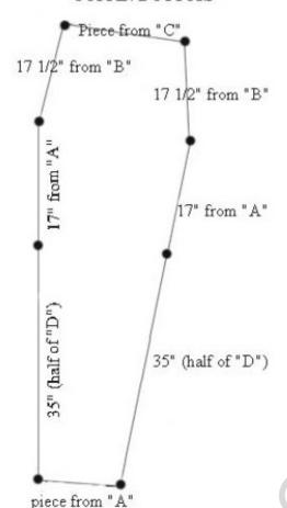
This sketch shows how to cut the A, B, C, and D pieces so they will fit around the coffin bottom.
