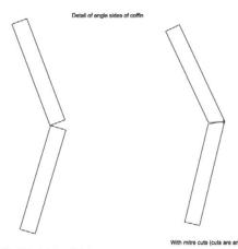
Without angled cuts where the sidewall segments meet each other, there will be a gap on the outside. The exact angle of the cut doesn't matter, as long as the two segments can touch on the outside. A gap on the inside is easier and neater to fill (with caulk, putty or epoxy) than the outside is.
