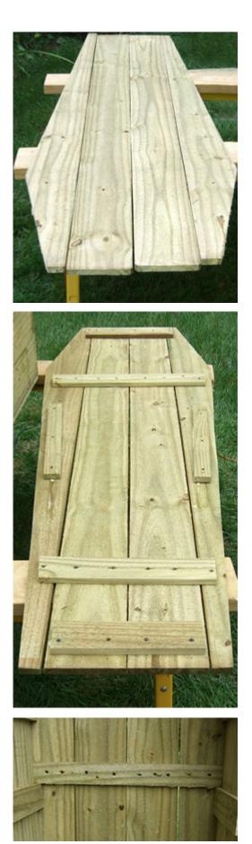
Boards #1, #4, #5 and #8 form the sides of the top and bottom of the coffin. These must be cut to achieve the toe-pincher angles. Marks were made two inches from one side on both the top and bottom edges. Another mark was made 16 inches from the top on the side opposite the other two marks. The marks were connected by a line which was used for the cuts. We ended up with two sets of four boards shaped like those in the picture on the right.
