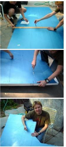
Here you can see us measuring and drawing our designs with a grease pencil. We cut the foam into thirds length wise, then 2 of the 3rds into more thirds, and the last 3rd in half. This gives us 8 pieces. Actually, we cut one of the pieces a little taller with it's top being the sides of the pieces cut in half. The foam we got came with some platic coating which we peeled off. Sometimes it would come off nicely and other times it would be a pain.
