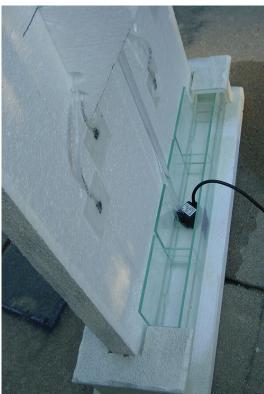
However, when it was first tried outside, wind moved the Styrofoam back and forth causing it to dig into the fins, so pieces were added between the fins. Holes were notched out of the bottom spacers to allow the water to flow back to the pump.
