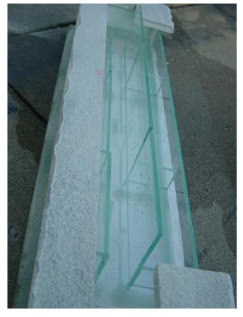
The back supports are higher to support the stone from falling backwards. If we were to build this tank again, we would use a solid piece going all the way across the tank, and the fins behind it, instead of cutting pieces to fit between the fins.
