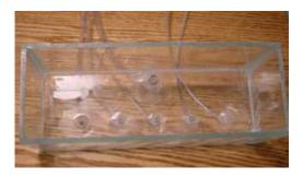
At first the tubes were placed inside the holes, but the water shot out of the holes and could not be contained. The upper tank has one  $\frac{1}{2}$ " feed tube and five  $\frac{1}{4}$ " tubes which feed the bullet holes.
