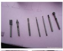
I use several different tips for my carving with the Dremel, depending on the look I'm going for or the size of the text or image I'm trying to carve. Since I'm using a plunge router with my Dremel, I am using the corded Dremel that has the plastic end that screws off. This is so the Dremel can then be screwed into the router attachment for stability.
