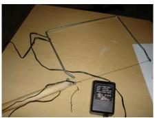
You can buy plug in types from other places like the Hot Wire Foam Factory... or you can make one yourself. I recently made one myself using Wolfstone's instructions and I LOVE it. Before, I was just using the battery operated one. The wire gets heated by the power source and glides through the foam like a knife through butter.
