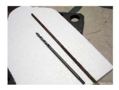
Drill bit and rebar -I just twist the drill bit by hand until only a little is left sticking out, being careful of the angle it's going in:
