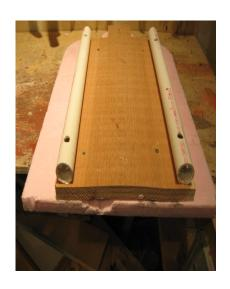
I then used a cedar board glued to the back of the stryofoam board to keep it stable in the wind. A couple of lengths of 1/2" PVC pipes screwed to the back. This allows a place to slide in your rebar. This rebar is pounded into the ground...to hold the thing up.
