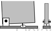
Here is a diagram of the setup. I used a small motor I had from a store display. This is about a 12 rpm motor but I replaced the 4 D cells it ran on with a 3vlt transfomer.
