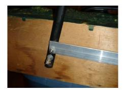
To start this project you will need to nail the two pieces of wood together to from an L shape. This L shape will be the platform to hold the grave up while it's moving. Next you want to drill a hole on L shape piece. This will hold the stake in place. You want the hole to be 6 inches from the end of the wood and 3 inches from the top.
