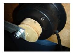
Take a scrap piece of ¾ inch ply wood and a hole saw and cut a 1 ½ inch diameter hole. The round scrap piece after cutting the hole is what you want to use to attach to the disco ball motor. Enlarge the hole if need ed to fit on to the shaft of the motor. Take the round piece and drill a 1/8 inch hole all the way through on the edge of the wood. Make sure before you drill the hole that the hole will line up with the hole in the shaft of the
