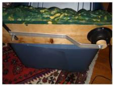
Take the piece of aluminum bar and you want to bend it so that it will form the shape of what it looks like in the picture. To bend the aluminum bar you can put it into a vice and use some force to bend it. Next you want to drill two holes on either end of the aluminum bar about a ½ inch in on both ends. The hole that will be attaching to the stake bolt should be off center while the hole for the motor bolt will be on center. Take a look at
