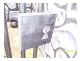
This is the custom made lock, made from wood and liquid nailed and drywall screwed onto PVC.
