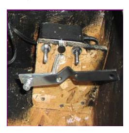
We had to make the bracket for the motor ourselves. It is simply (1) L-shaped bracket, filed down on one end to fit inside the shaft of the rotisserie motor, and (1) flat metal mounting plate, cut to the appropriate length and bent in the middle. (See photo).
