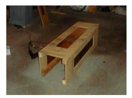
Cut 2x3's into 4 foot lengths. Cut 1/2" plywood into 15" widths, 4 feet high. Cut out rectangle from center of each, measure twice the width of 1x5 from bottom and top, and 4" in from the sides. Cut 1/4" plywood to just larger than these holes. Using construction adhesive, glue 1/4" plywood to **inside** of each 1/2" piece.
