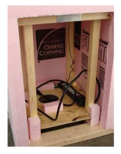
I left one sheet of foam off of the bottom so that I could have access to the bottom space. Later I added a sub woofer and power strip in this space. When most of the foam was glued and in place, it was time to start shaping it up. I used a free form hot wire cutter to remove large chunks out of the foam to create the angle.
