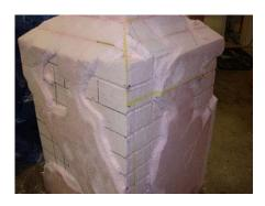
Marking the lines for the brick wasn't as easy as I had hoped. I made a template of a real brick with some thin cardboard.
