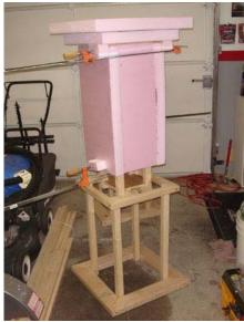
Once the frame was built it was time to add the foam. Using a mixture of Liquid Nails, wood screws, gorilla glue and great stuff, I was able to create the basic shape. Bar clamps worked well to keep the foam in place while the glue set.
