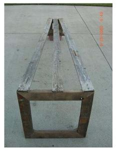
Put the 2' square on it's side on the ground and then get the 1' square and make it 6" off the ground. I used a brick and a 2x4 (you can see it in the picture a little bit). Get an 8' 1x4 (part of the free fence I found on the side of the road) and screw it to both the top and bottom pieces. Now put the edge pieces on and make these tilt inward at the top. Screw them down and do this on the two sides that touches this side. Leave the front side open because we will need that open for later.
