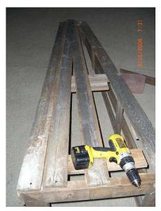
After you have screwed on the support boards, the door support boards, and the pipes, it is now time to start filling it in. Get another 1x4 and lay it down on the inside of the outside boards. Let this board tilt in the same like the two out side boards.
