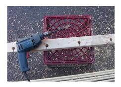
Using your drill with a 5/8" drill bit (I suggest using a speed bore bit, as pictured, to speed things up), drill the holes where you marked(remember the mark is the center of the hole, so your drill bit goes there). If you want to speed this up you can mark one board, and clamp a few together while drilling to do more than one length at a time).
