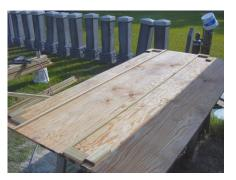
A simple jig is made for panel assembly. For the creation of this jig, scrap pieces of wood are nailed in position marking the maximum location of each corner of the panel sections. Long, thinner strips of wood are nailed in place to hold the vertical pieces at the proper height in relation to the top and bottom plates (ripped during the previous step.)
