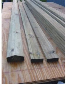
Basic sawing operations are required to prepare the dimensional pressure treated lumber.
