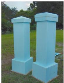
This photo shows a rough shaped post cap (left) and a post cap assembly prior to rough shaping.
