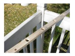
I drilled holes in two 8 foot pieces of 1x2 wood. Their are 16 holes 6 inches apart (3 inches in from each end) and 0.875 (7/8) inch in diameter.
