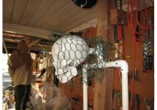
After that, I just started cutting pieces of chicken wire and securing it to the framework with zip ties.
