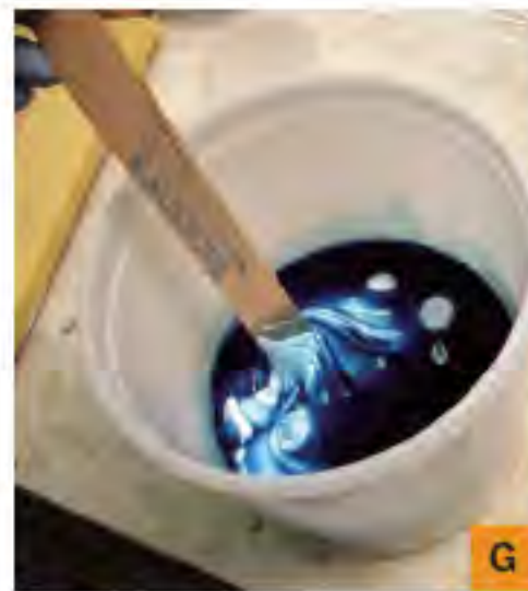
Fig. G: The silicone before mixing. Fig H: The silicone after mixing. If you see any white streaks, you're not nearly done. Fig I: Pouring the silicone. You should pour thinner than this, unless you have an evacuator to put the mold into immediately afterwards (like I did).
