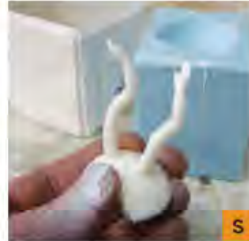
Fig. Q: Pouring the resin. Fig. R: The main casting unpacked from the mold. Fig. S: The arms removed from their mold. Fig. T: The finished casting, cleaned up, glued together, and painted with primer.
