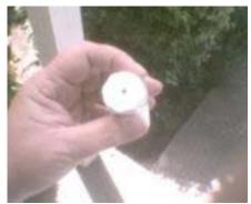
I drilled a small hole in the end cap and then I took some plastic putty kneaded it and filled the end cap with it. Before the plastic putty set-up I inserted the needle into the end cap business end into the putty .
