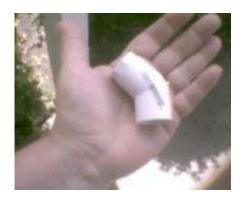
I just used a 45% PVC joint with and end cap to fit, the size I picked was 1/2" Joint Connector and End Cap.
