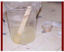
Step 5: **MOST IMPORTANT**. Allow the melted gelatin to cool for between 5 - 10 minutes depending on the melted temperature, until the gelatin is only warm to the touch but not gelled yet. The hotter the gelatin is when it is foamed the more translucent the foam will be but it will have a coarser and uneven cell structure with heavier body.
