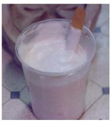
Step 7: Once it has stopped, stir the foam to refine the large bubbles until an even cell structure is reached. It should be at a Meringue consistency. It is possible to reheat the foam to allow the foam to pour into a mold or to inject. Some do this anyway and claim a much better foam. They heat for about 30 seconds only and stir again.
