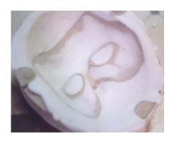
Step 10: You can tell that the foam has gelled the same way that you tell if Foam Latex has gelled. Poke the runoff and if the runoff bounces back its ready. Remove the mold from the freezer and peel the flashing from the outside of the mold. This will keep the foam from sticking to the mold while opening. A screwdriver will help in the initial opening but it should be done slowly in much the same way a Foam Latex mold is opened. Once open, powder the inside of the appliance.
