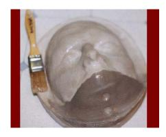
Step 2: Apply release to the Positive side of the mold. It is optional whether this side is heated or chilled in the freezer prior to foaming. If chilled it should only be cold to the touch and not frozen. The goal here is only to speed up the gelling time. Experience will dictate what is appropriate.
