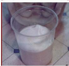
Step 6: Add the dissolved Part B to Part A while stirring. It will immediately begin to foam. Stop stirring at this point and allow the foam to rise.
