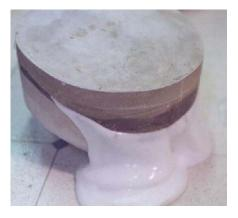
Step 9: Close the molds immediately after filling and either clamp or stand on the molds to insure a thin blending edge. Place the closed molds into a freezer to gel. Depending on the size of the mold and its temperature it will take between 30 minutes to an hour before you can remove the appliance. The longer the better but still faster than baking Foam Latex.
