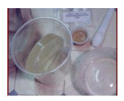
Step 4: Remove Part A from its container and place it in the large container provided. Melt the Gelatin Base (Part A) in a microwave oven for **no more than 1.5 - 2 minutes**. Do not overheat (boil). It is better to remove early and allow the unmelted part to slowly dissolve while stirring.
