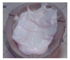
Step 8: Load your molds. Spatulate the foam into the warm negative mold and close immediately. This step is the same as for Foam Latex. Be careful not to trap large air bubbles. You can also inject the foam but the mold needs to be warm.
