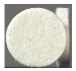
The first step was grinding away the seam using a Dremel felt polishing wheel.
