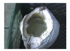
We rolled the mold around quickly, making sure to get the eyes, ears, chin, and other detail parts covered, and then put the molds down so the foam could expand.
