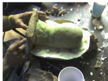
You will want to create some wedges out of clay to put on top of the plaster... these will make pry points if you have any problems separating the two halves of your mold later. Unfortunately, I didn't get any pictures of this part, but you can see them sticking out in the picture below. The wedges should go about 2/3 of the way between the outside of your mold and the item you are casting, but definitely not touching the item you are casting.
