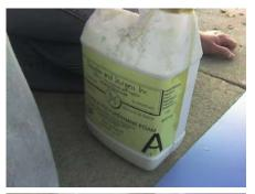
Bryan used a 2 to 1 foam from <u>Douglas and Sturgess</u> It takes less than 5 minutes to fully expand, and then (mostly) cures in 20 minutes.
