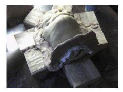
When you have the blocks positioned correctly, you can start to make your wall. You want to create a flat surface all the way around the item you are casting, and make sure that the clay goes all the way to the edge/surface of what you are casting. We used tongue depressors for the most part, and then some clay working tools for the fine detail. Don't forget to make a wall across the bottom edge as well.
