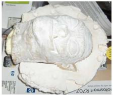
And then... the release! Turns out I was able to separate the two halves of the mold by hand, so the pry points were not necessary.
