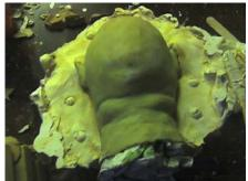
Once the plaster has set firmly, turn the mold over and remove the clay and blocks.
