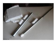
Push and twist a thin-walled pipe into a chunk of Styrofoam to create 'cylinders' that will be used for the fingers. Use the piece of rebar to pop them out from the pipe.
