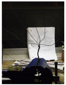
The first thing to do is to cut 10 pieces of heavy duty wire measuring about 50" long each. I don't know how to measure the gauge of the wire I'm using but it is very similar to coat hanger wire. Separate the wire into two piles, each will be an arm, and guesstimate where you'd like the wrist to be and using two sets of pliers, twist the wires together tightly for about 3" of twist to guarantee it's secure.
