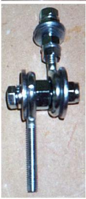
Before our dummy can begin to take shape, we will need to assemble all 12 of his joints. This will entail preparing the pipe cap fittings with the necessary 5/16" hole in the center of each. Also you need to assemble the joints and attach them to each cap. Here you can see how each section goes together.
