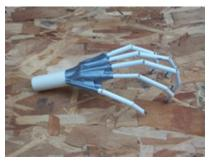
Once all the fingers. are complete attach them to the PVC by sliding the wire through the holes. The L shape bend should lock them in place. Using your own hand as a guide space the knuckles of the hand to roughly the same as yours. Then tape them in place with duct tape or masking tape.
