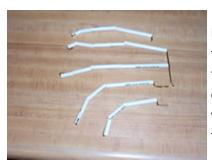
Next you need to make the fingers. I just take the bic pens and hold them up to my hands. I start at my wrist to the first knuckle. Then cut the pen to length. Then joint to joint and so on. Once all the joints of one finger are cut slide them over a coat hanger. Bend the end that will be the finger tip and crimp it with pliers. On the other end bend the wire in a L shape and cut the wire..
