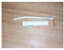
Start by taking a piece of PVC about 5 or so inches long and using a hammer smash the end. It cant be seen in this picture but I cut a noch out of it about a inch down the length. This just makes it easier to install the fingers. You will need to drill small holes into the PVC for the fingers. I drill four holes in a row and then one for the thumb about a 1/2 inch lower.
