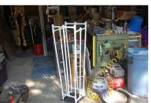
I also put 4 of my 1.5 inch pieces in place in 2 assemblies as these will go together much like the base pieces did. Take the two assemblies with the 1.5" stubs and attach them to the three on one side that are all the same height. repeat for the opposite side. the stubs will be pointing up so you can take the remaining two assemblies and attach them to the
