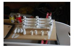
Next pull out 12 t fittings the 3.5" pieces of PVC, the 2 " pieces of PVC and the four caps. take 3 T's and 2 -3.5" pieces and assemble as shown here. have 4 of he 1.5 " pieces standing by.
