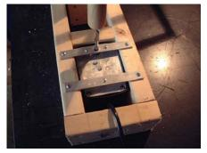
Drill two holes into the center of the 30" pieces and mount the mechanism to the rail with bolts, washers and nuts (fig. 8). Use a metal file to round off any sharp edges on the aluminum.
