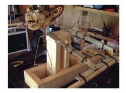
Cut a wire coat hanger as long as you can make and use it to form the linkage guard, this will prevent your linkage from getting tangled with the robes and provides the spine for your ghoul (fig. 10). (Instead of cutting off the excess wire, I attached it to the head of my ghoul for a bit of secondary action. I also used another length of wire to form the sternum.)
