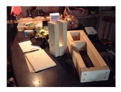
Cut two additional blocks at 3 1/4" and wedge them into the box (fig. 3), these will act as the upright and servo tray supports. Cut two 10 1/2" inch pieces and a 5" piece of the 2x4", screw them to the front 3 1/4" block as shown to serve as the upright support.
