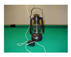
Here is a standard lantern available at any hardware store. I cut off the bottom, installed a flicker circuit, a 9v battery eliminator, a bulb socket, and bulb. I then used a plastic cup and some fiberglass to seal up the lantern. A little black and brown paint and here is the old looking lantern
