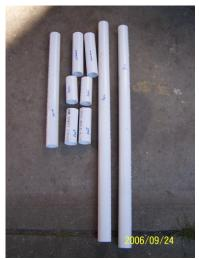
He's made of a simple PVC frame. Here you can see I have all the parts marked and cut. I used 1 1/4" PVC. All pieces are cut to what ever length you need for the size wanted.
