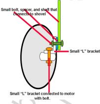
Here is a diagram of how the motor is attached to the shovel
