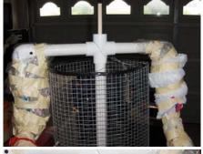
Here is a closer look of the upper connections. You can see on the left shoulder a screw. I secured the joints with screws to hold it together better.
