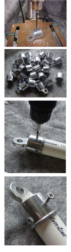
I used the drill press to add holes on all 4 sides
