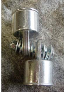
I used the same "spring tension" system to bolt the "bones" together and create working hinges / joints
