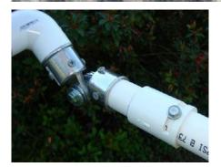
The pin and slot rotators are made with a 1' PVC coupling.
