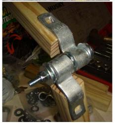
My plan is to build an articulated human frame with off the shelf parts. In this case I went with the spring tension method to hold the joints stiff after posing the figure
