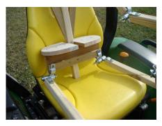
I used 2"x2" treated pine as the primary material, but also there is a few feet of 1" x 2" pine and 1" x 4" and 3/4" plywood...It took me 2 hours to figure out what parts to buy at Home Depot and 6 hours to design/build the standing form...I think the next one I build will take less than 3 hours
