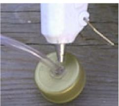
Start by removing the plastic seal (ours was blue) from inside the lid with needle-nose pliers, the glue won't stick to it very well. Now carefully drill a hole the same diameter as your clear tubing through the center of the cap. Remove any plastic debris from the drilling, then lightly sand both the inside and outside the cap around the hole to help the glue stick to the plastic better. An emery board works great.
