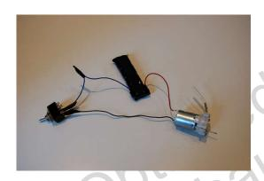
Set up a simple circuit with your switch, but don't test your pump just yet. It isn't necessarily bad for the motor to run a dry pump, but it's not something you really need to risk.
