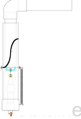
As the piston pushes forward, the metal bar rides in the spiral shaped slot. This causes the 1.5 inch pipe to twist and raise. It does this with considerable force. I fitted an elbow and another 12 inch piece of 1.5" PVC pipe to the end of the inner PVC to form the arm. It swings it with enough force that I decided to get some thin wall PVC (instead of the schedule 40 I used everywhere else) so that it was lightweight enough that if it hit anyone, it would not hurt them.
