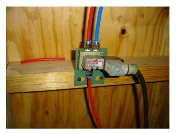
Do you see the little connectors I am using? Those are 'quick-connects' or 'instant-fittings', depending on where you buy them. I paid 63 cents each for those that go straight out from the solenoid. They are 1/8" NPT threads and adapt to 1/4" polyethylene tubing. The tubing costs \$7.50/100' roll.
