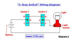
So, how does this work? Let's say that Switch 1 is at the bottom of a stairway and Switch 2 is at the top. Suppose Switch 1 is in a 'down' position (B & C connected) and Switch 2 is in an 'up' position (D & E connected). The light bulb is off. Now someone comes to the bottom of the stairs and flips Switch 1 up'.
