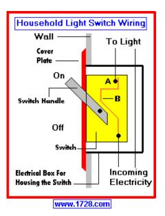
This type of switch (having a lever which "flips" it on and off) is called a toggle switch.
