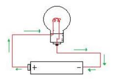
Notice that the power flows from the "+" (POSITIVE) side of the battery, through the light bulb and back into the "-" (NEGATIVE) side of the battery.
