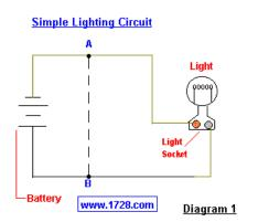
Diagram number 1 illustrates an extremely simple circuit. (For the moment, ignore the dotted line and the points A and B). The battery is represented by 4 lines (the longer line being positive and the shorter one negative). Starting from the negative end of the battery, electrons "circle" through one wire, pass through the light bulb, pass through the other wire and then return to the battery thereby completing the circuit. See? Quite simple.
