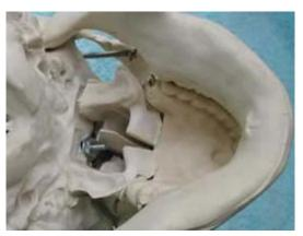
Using the #6 screw, nut and washer, mount the servo bracket in the Bucky skull. Tighten securely but don't over tighten as it might bend the bracket.
