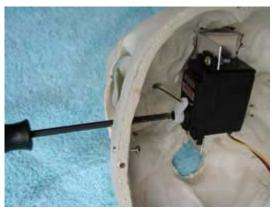
At some point, you're probably going to need to adjust the position of the servo horn on the servo. I recommend drilling a small hole in the side of the skull, as shown left, to accommodate a small phillips screwdriver. Be careful when drilling the hole so as not to slip and drill out the center core of the servo (please don't ask me how I know about this).
