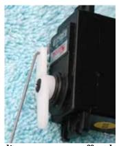
Next, using a pair of long nose pliers, create an offset bend, as shown left, in one end of a 6" piece of the music wire. Attach it to the outer hole in the servo horn as shown right.
