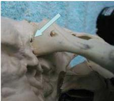
Bucky's jaw is held in place by a pair of springs. We need to install a permanent pivot for the jaw and also eliminate the springs because they are too much mechanical resistance for the servo. We'll use the cable ties as our pivot.
