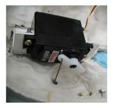
Feed the wire through the hole and install the servo in the bracket using the #4/40 screws and nuts. I find that using just two screws will hold it securely in place.
