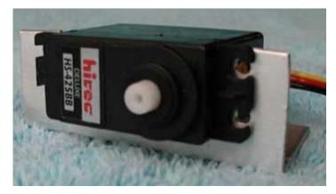
Using the appropriate tools (hack saw, tin snips, file, etc.) cut an opening in one side of the aluminum angle to accommodate the servo. Be sure to leave some of the "angle" to maintain strength. Drill holes to match the servo mount for 4/40 screws. This will be our servo bracket.
