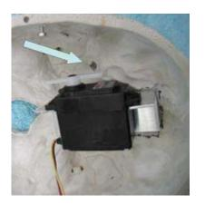
While holding the servo in place, make a mark on the skull in line with the two points described above (left). Drill a 1/4" hole in the skull at this mark. If you were really good (lucky?), the hole will line up perfectly between the two points, if not, you'll have to "modify" the hole slightly to be in line.
