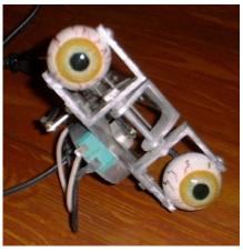
Near the center of this picture you can see the crank for the left/right motor
