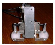
Bottom view showing main frame, eye mounts, and linkage for left/right movement. Control arms mounted on back of eyes are made from aluminum angle. L/R movement linkage works just like the steering in a car (except rack and pinion) the crank controls one side, a tie rod controls the other
