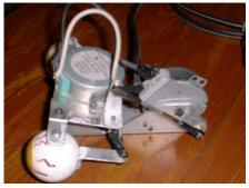
Here you can see the up/down motor, crank, link, and control arm.
