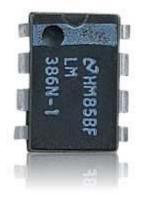
LM386 Low Voltage Audio Power Amplifier (8-Pin DIP)
